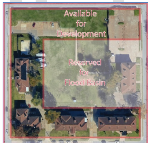
Figure 3 Approximately 2.6 acres of the 4.4 acre site is offered for redevelopment. The center of the 4.4 acre site will be reserved for a future flood control basin. The exterior portion of the 4.4 acre site would be the focus for the redevelopment effort.
